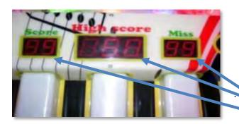
When in programming mode the center display will display the current Bonus Score setting. The two other displays will display 99.
