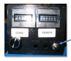
Press and hold the program button directly below the Ticket counter for 10 seconds to enter into programming mode.
