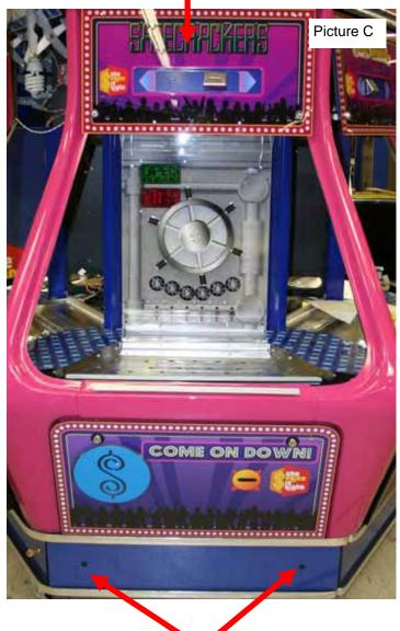
Remove these two bolts to access AC Power Cord and AC ON/OFF Power Switch. See Picture A and B for Close Up.
