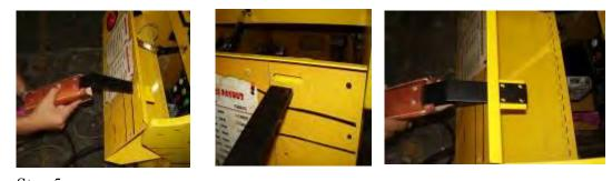
Step 5, Screw the 4 supplied L bolts to hold the bracket as shown below,
