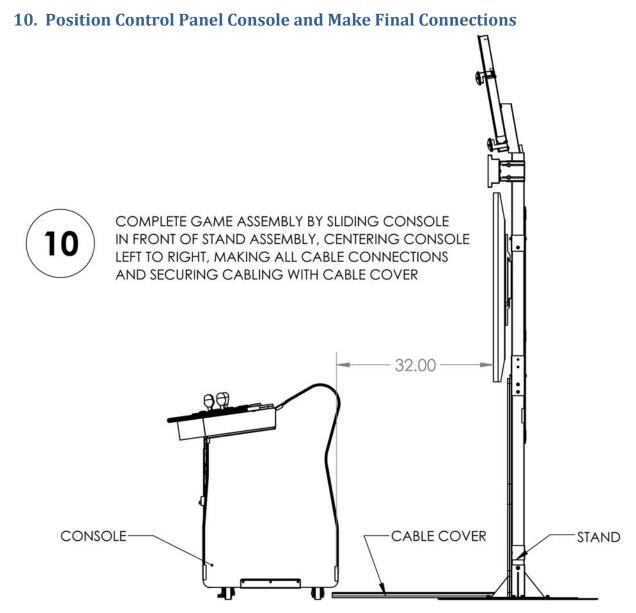
Connect HDMI cable from display to PC HDMI port. Connect RJ-45 cable from LED Ribbon to LED Sending Card. \*\*\*DO NOT CONNECT TO PC\*\*\*
