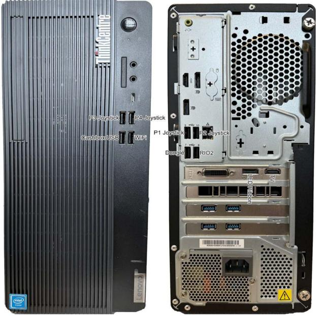
\*Note – TV must be connected by an HDMI cable. Do not use an HDMI adapter.
