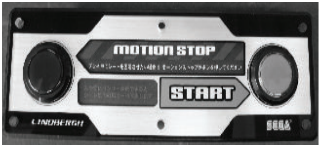
FIG. 6-5e MOTION STOP BUTTON guide attached to the SW PLATE.
