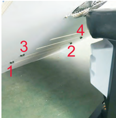
Remove screws from back door that hold the light box
